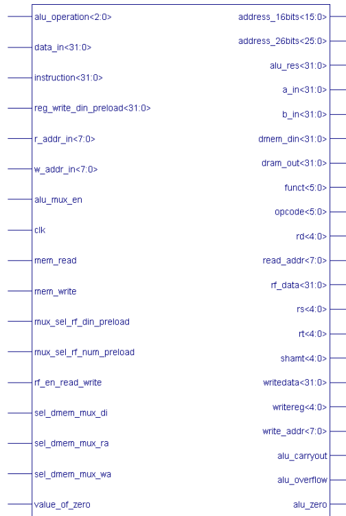
Figure B.26 Resulting top level RTL symbol for the datapath section for LW and SW instructions.
